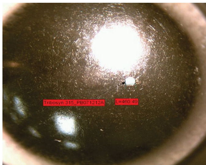
Figure 4. A ball bearing protected with a grease made using Tribosyn 315 AN base oil showed only a small wear scar (small white spot indicated by black arrow).
