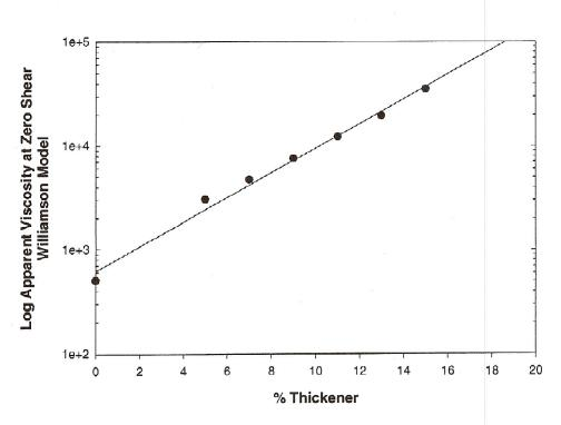
A first order linear regression of the data resulted in the following coefficients: slope of 0.1186, y-intercept equal to 2.792 (619 mPas) and a correlation coefficient of 0.994.
